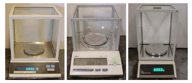
Be aware that these balances are somewhat delicate and very sensitive. Do not remove the plastic guard around each. While it may not always be practical to do so, it is good practice to stick with the same balance during any particular experiment. Pictured are the three models of analytical balances that we use in the General Chemistry. During the first lab, your TA will demonstrate the various idiosyncrasies of each! When doing any weighing, please observe the following:
